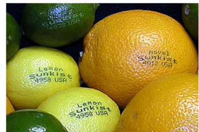
New laser labeling technology uses a carbon dioxide laser beam to etch product information into the first few outer cells of the peel of a fruit or vegetable. Some say the system could replace sticky produce labels.
